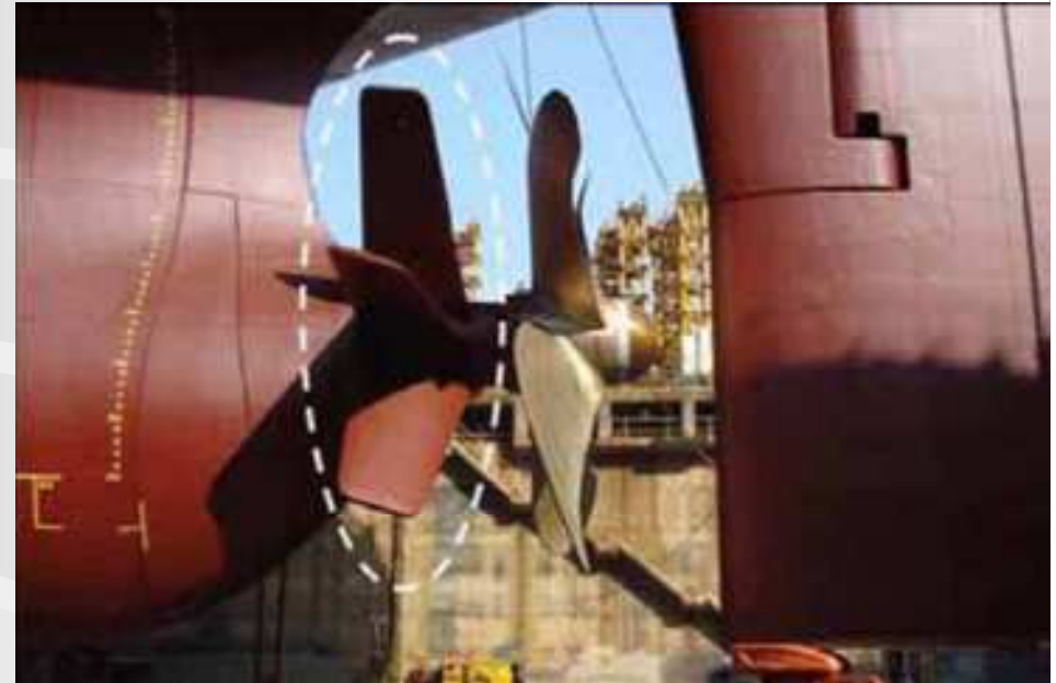
Pre-Swirl Stator (Daewoo Shipbuilding & Marine Engineering)
